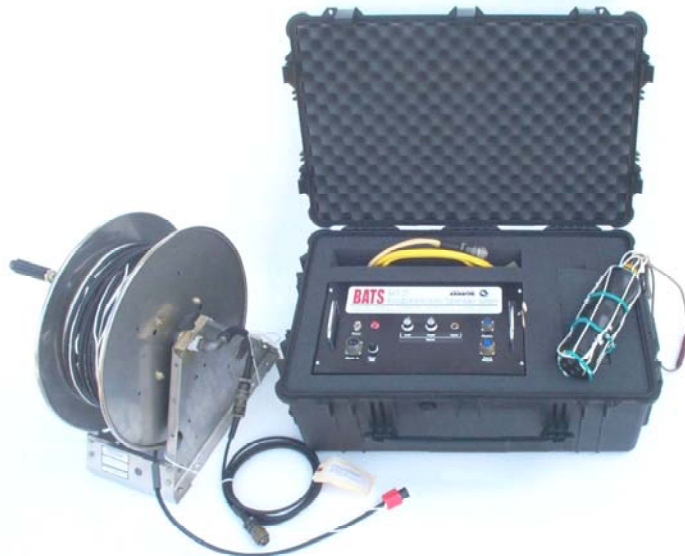
Fig. 3. Typical configuration of a Broadband Acoustic Transmission
